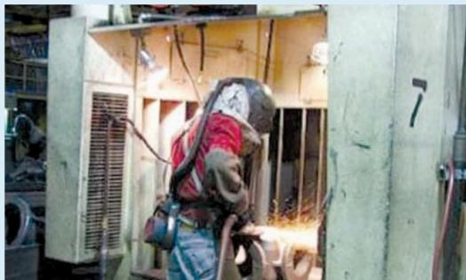
booth that draws air away from the worker so he doesn't breathe the dust created by the grinding. This method can be used in material handling (such as bag dumping), mixing operations, rock crushing, and other dust-producing activities.
